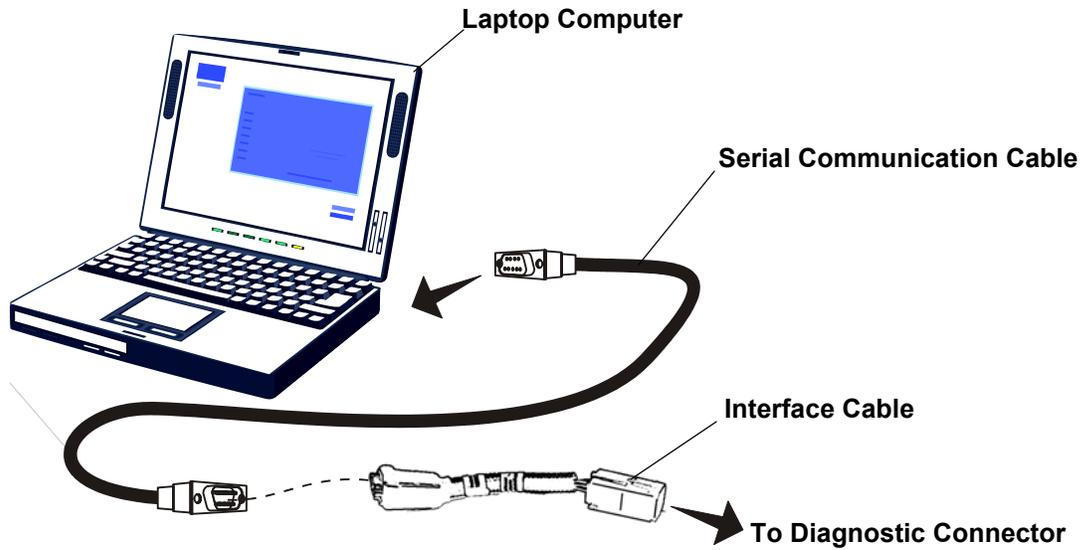
For connection to a PDA, use kit PN 2U1E-6K947-AA. Connect as shown below:
