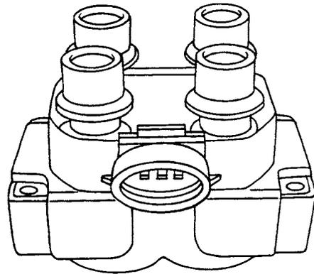
The primary coils in the coil pack are triggered by the "ignition coil feed#1" and ignition coil feed #2" signals from the EPM.
