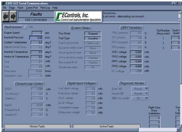
The Injector Kill mode is used to disable individual fuel injectors. If the Injector Kill mode is selected with the engine running below 1000 RPM, the minimum throttle command will lock into the position it was in when the test mode was entered. If the Injector Kill mode is selected with the engine running above 1000 RPM, the throttle will continue to operate normally.
