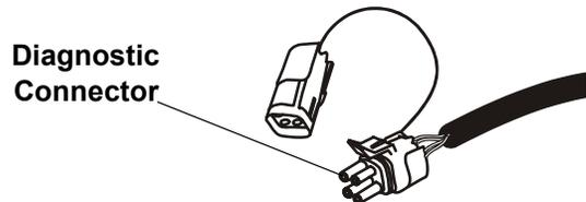
The MIL displays three digit codes by flashing the first digit, pausing, then flashing the second digit, pausing, and then flashing the third digit. There will be a long pause between codes. For example, a code 143 would be one flash followed by four flashes followed by three flashes.
