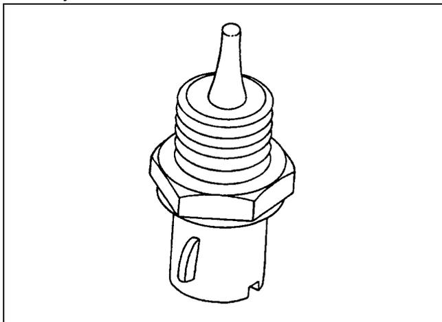
After engine start-up, the temperature should rise steadily to about 85°C (185°F). It then stabilizes when the thermostat opens. If the engine has not been run for several hours (overnight), the engine coolant temperature and intake air temperature displays should be close to each other. A fault in the engine coolant sensor circuit will set a DTC 221 or DTC 222.
