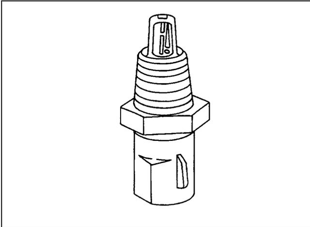
The diagnostic software can be used to display the temperature of the air entering the engine. The temperature should read close to the ambient air temperature when the engine is cold, and rise as engine compartment temperature increases. If the engine has not been run for several hours (overnight), the IAT sensor temperature and engine coolant temperature should read close to each other. A failure in the IAT sensor circuit will set DTC 211 or DTC 212.
