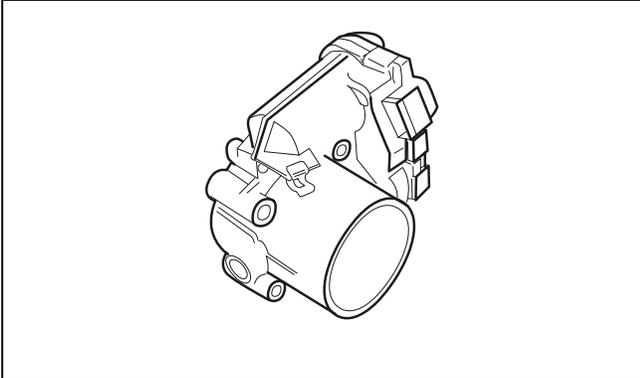
The Electronic Actuator also acts as an idle air control (IAC) valve. Changes in engine load are detected by the EPM by comparing manifold absolute pressure (MAP) with throttle position. When the EPM detects a change in engine load, it can adjust idle speed by changing the PWM signal to the actuator.
