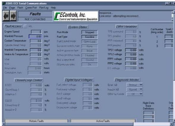
The Spark Kill diagnostic mode allows the technician to disable the ignition on individual cylinders. If the Spark Kill diagnostic mode is selected with the engine running below 1000 RPM, the minimum throttle command will lock into the position it was in when the test mode was entered. If the Spark System Test mode is selected with the engine running above 1000 RPM, the throttle will continue to operate normally.
