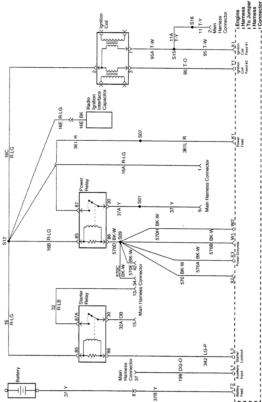
ECM to EPM Engine Wiring Diagram (2 of 5)
