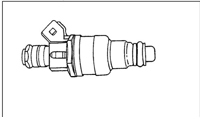
The fuel is injected under pressure in a conical spray pattern at the opening of the intake valve. Excess fuel
