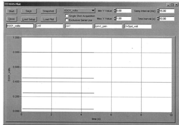
Recording the values and voltages can be a very useful tool while diagnosing engine problems. The FORD diagnostic software includes real time **plotting** and real time **logging** capabilities. These features enhance the ability to diagnose and repair possible problems with the FORD system. Both plotting and logging allows the user to record, in real time, any variable that can be seen in the FPP\_Dis software. In order to record variables, the FPP\_Dis software must be "Connected" to the EPM.
