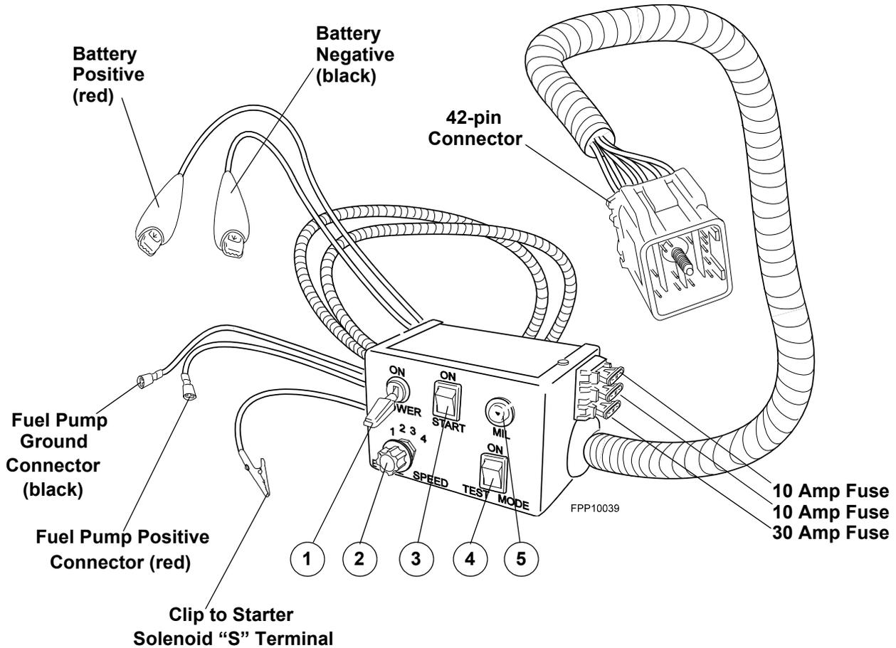
1. Power Switch: Flip to ON to energize system.
