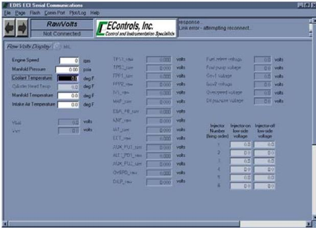
The RAW VOLTS screen shows actual voltage readings from various circuits.
