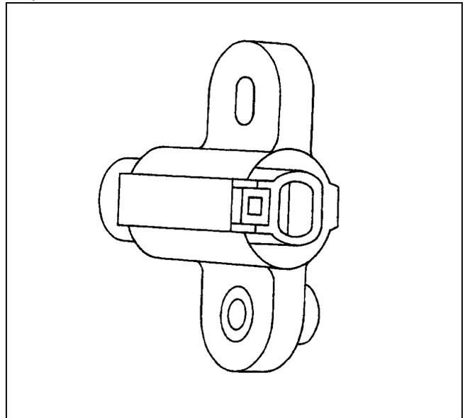
**Engine Coolant Temperature (ECT) Sensor**
