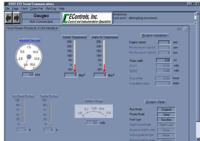
Most applicable sensor and actuator values are displayed on the Gauges Screen. The display shows the voltage the FORD system EPM is reading and, for sensors, the sensor value in engineering units.
